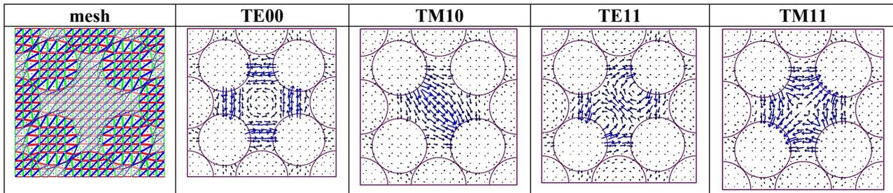
Figure 4. Schematic representation of the perfectly confined eigen-mode spectra.
